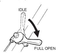
Figure 9. Throttle Lever (Full Open)
